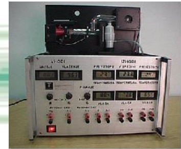
Air conditioning pilot plant
